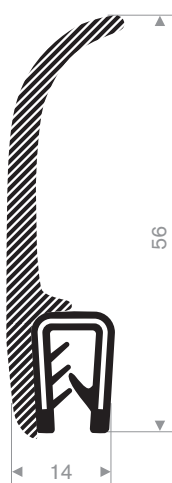
245.00.876 pvc + mosrubber klembereik 1-3 mm
