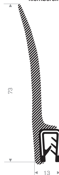
245.00.877 pvc + mosrubber klembereik 1-2 mm
