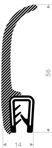
245.00.876 pvc + mosrubber klembereik 1-3 mm
